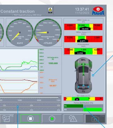
Display of vehicle's power distribution and power flow
