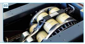
Eddy-current brake for performance measurement and load simulation:
