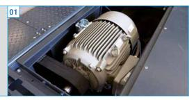
E-motor for all-wheel synchronisation: tracking acceleration on the non-driven axle
