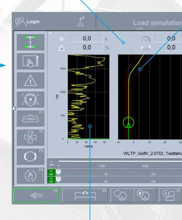
Cycle time, gradient, current speed and distance covered can be read on the display
